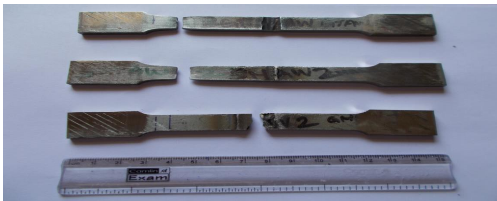
Figure 8: Fractured Sample in Tensile Test
