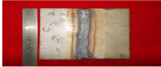
Figure 3: Welded Specimen by GTAW
