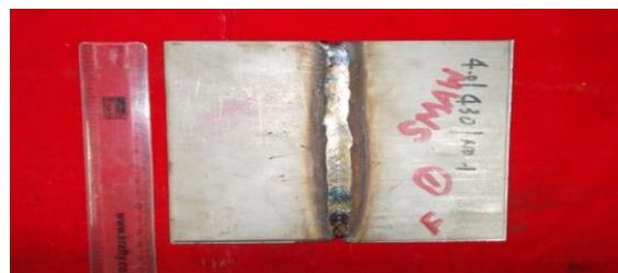
Figure 2: Welded Specimen by SMAW
